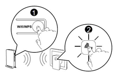
Please press and hold Wifi/WPS button on the router first for 5 seconds and then press the Amber switch on the WS320 (the Amber light will begin to flash).
