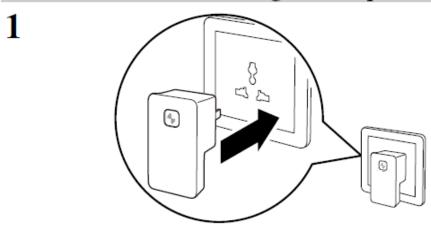
Connect the WS320 to a power socket and wait for Amber light.
