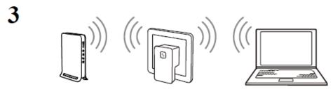
Wait until the flashing Amber light changes to solid green (generally about 20s and less than 120s) and you are set up and ready to move the WS320 to its final location.
